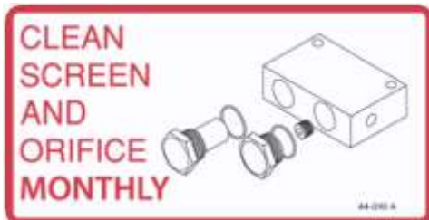
44-090, DECAL, WARNING MANIFOLD MAINTENANCE
