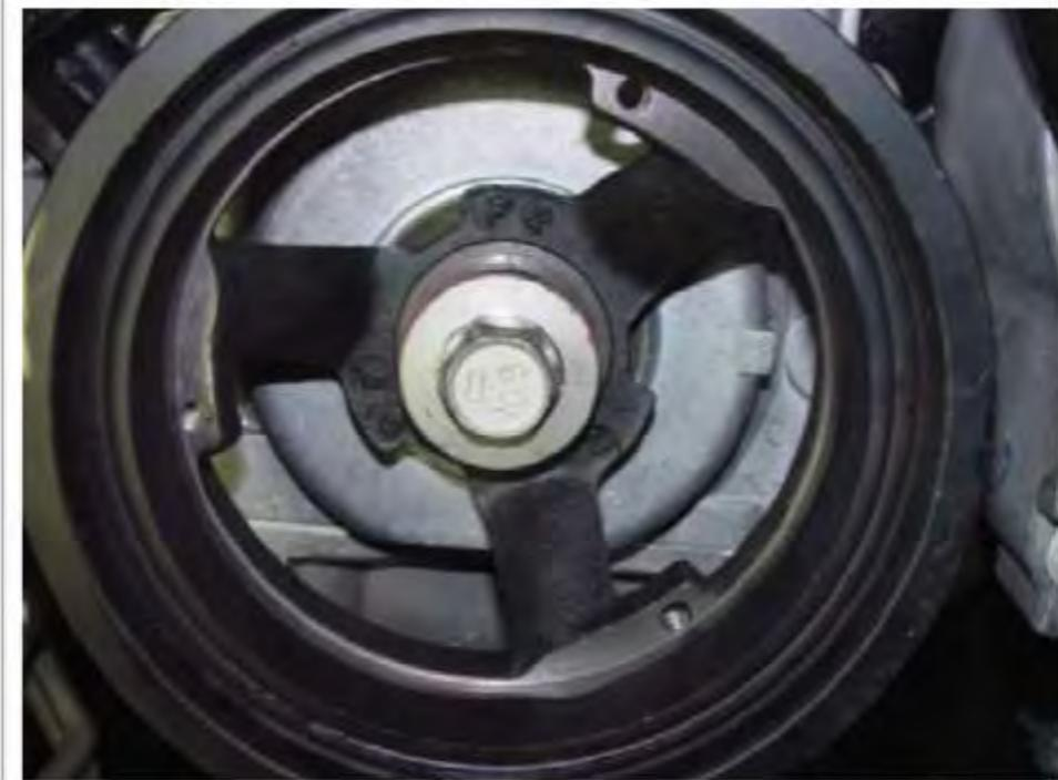
20. Use **OLD** balancer bolt and tighten to 240 ft lb torque. Remove bolt, wipe balancer clean and install new bolt. **DO NOT** use any lubricant, Loc-Tite, etc., of any kind. Tighten bolt to 37 ft lb.
