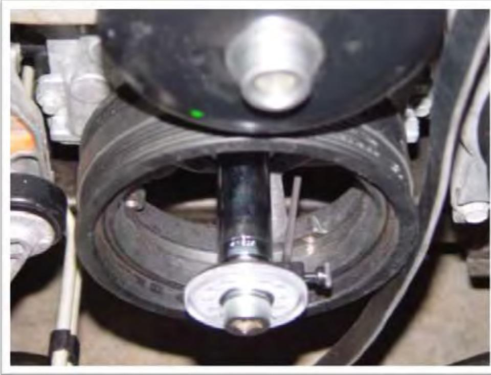
21. Use torque angle meter to further tighten to new bolt another 140°. **Note that the measuring face of the meter must be secured from turning and set to zero before further tightening the bolt**
