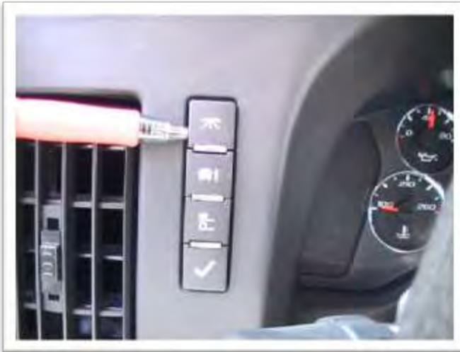
5. Press the top button to the left of the instrument cluster until the tachometer is displayed.
