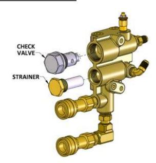
**NOTE:** New o-rings must be installed **anytime** the check valve is removed.
