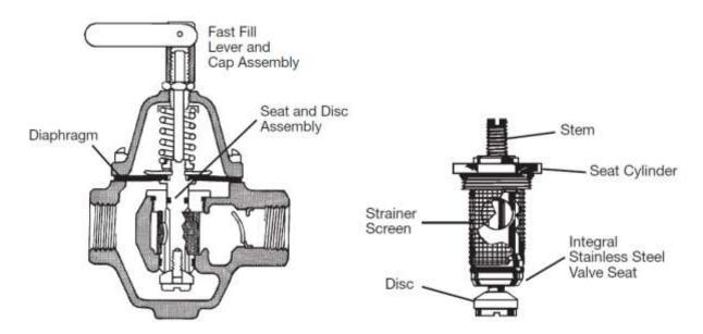
The second stainless steel mesh screen is located inside the inlet pressure regulator. Inspect and clean at least once a month. Hard water deposits can build and reduce water flow.
