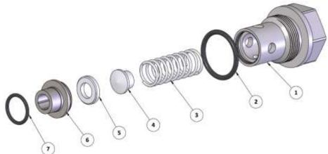
23-063 ASSEMBLY, CHECK VALVE MANIFOLD
