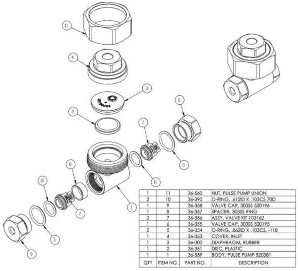
The chemical pump should be rebuilt every **500 hours.** This involves changing the diaphragm and plastic disc, check valves, and inspecting the disk. **DO NOT** attempt to reuse O-rings after the check valves have been removed. Replace all O-rings when servicing check valves.
