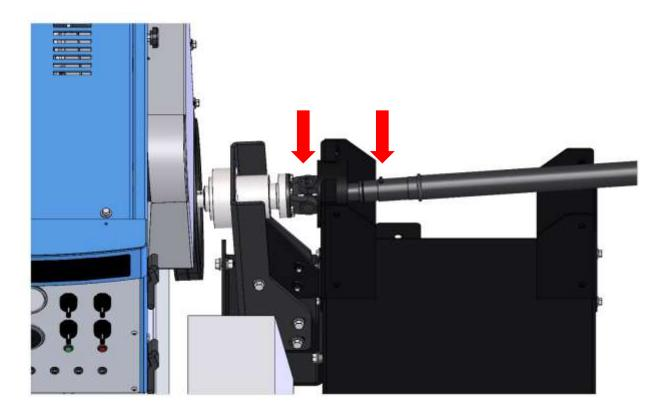
The drive shaft splines should also be lubricated with the same grease as the zerk fittings.
